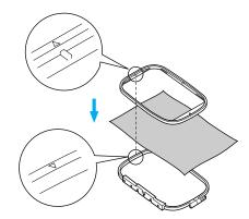
Tighten the adjustment screw by hand just enough to secure the fabric.
